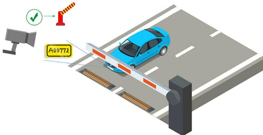
Figure 12-2 Example: Barrier Opened Automatically for Vehicle in Vehicle List
